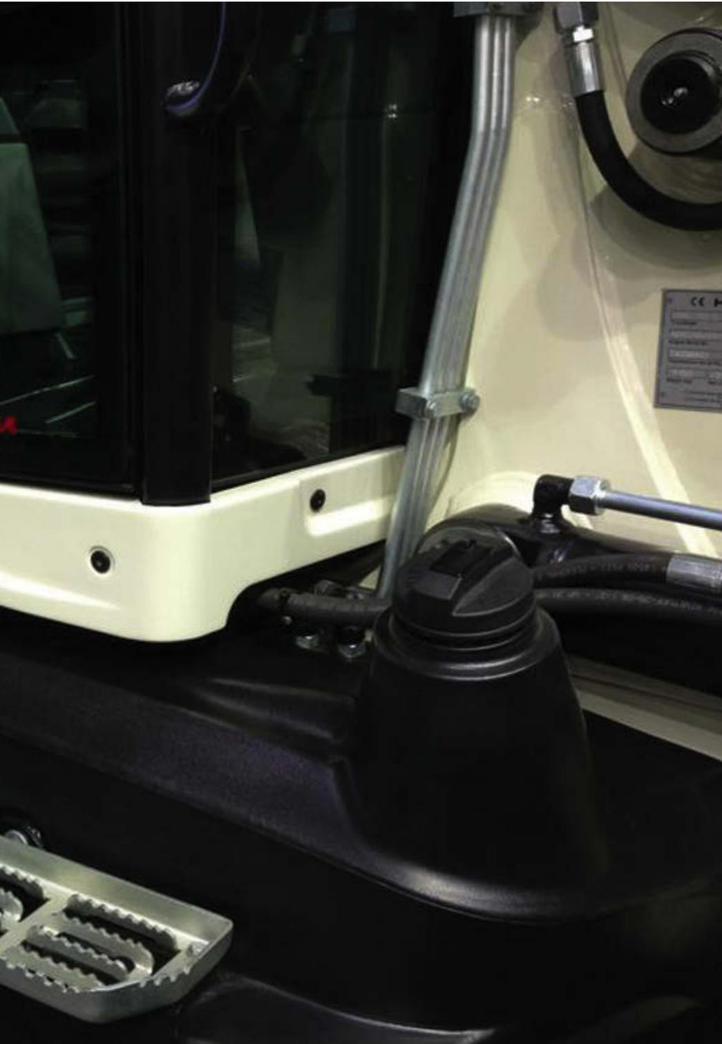
LEFT: Hidromek's Maestro show model at Bauma featured its serial pDCPD fenders and cabin fittings
